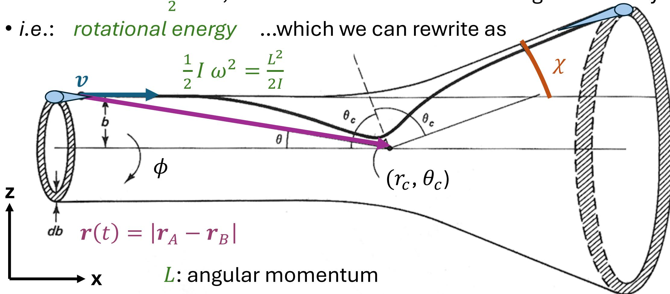
$$E = \frac{1}{2}\mu\dot{r}^2 + \frac{1}{2}\mu r^2\dot{\theta}^2 + U(r) \quad \text{we can rewrite as}$$
